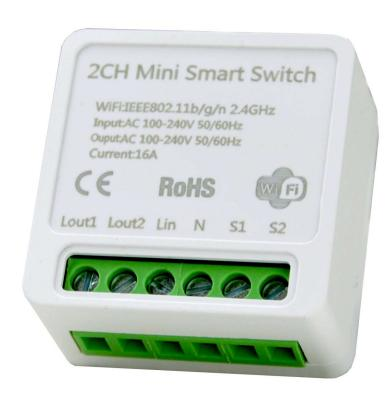
L-in / N -Connect 110..240VAC input power supply
