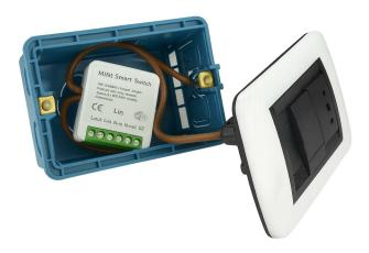
L-in / N-in -Connect 110..240VAC input power supplyL-out / N-out-Connect the 110..240VAC device to be controlledS1 / S2-Connect local switch
